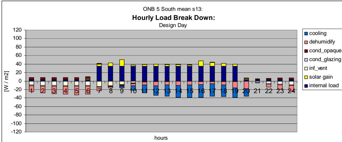
**Graph 65: hourly gains and losses for ONB s13 (extended nocturnal ventilation)**
