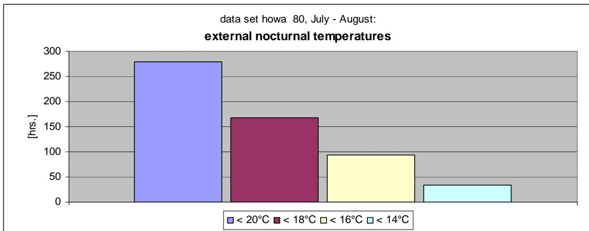
**Graph 46: Amount of hours with external nocturnal temperatures under-running various limits, data set "howa 80"**
