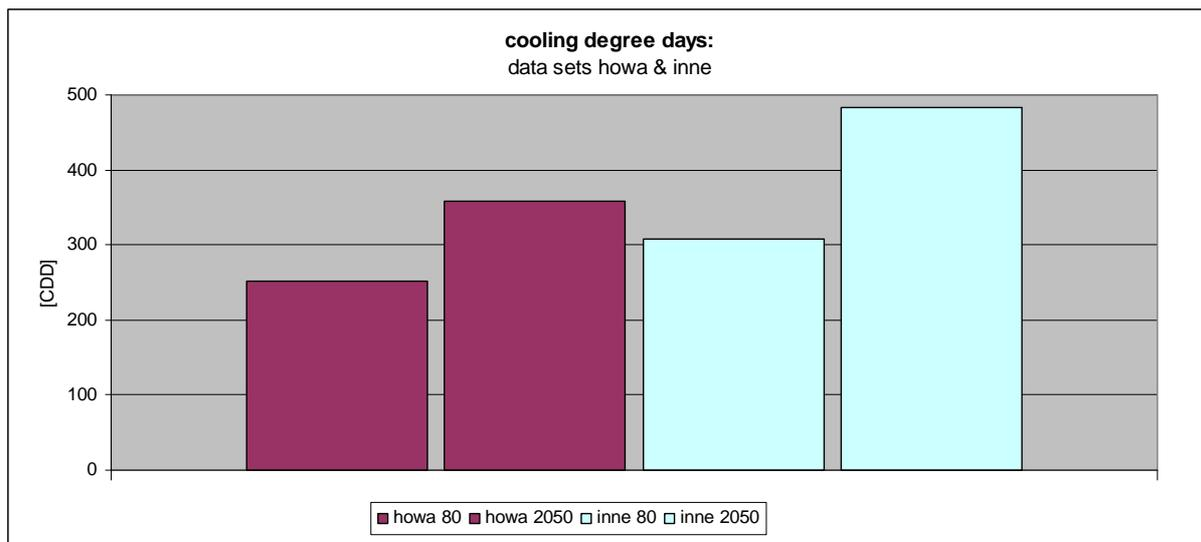
**Graph 5: Cooling Degree days of data set “howa 80” and “howa 2050 (Main Weather Station) and “inne 80” and “inne 2050” (CBD)**
