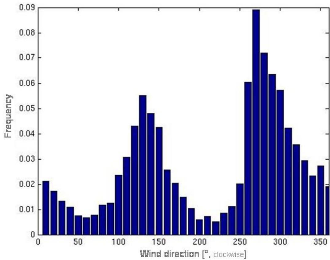
**Graph 48: statistical distribution of wind directions (indication of degrees clockwise) for 6:00 a.m.**
