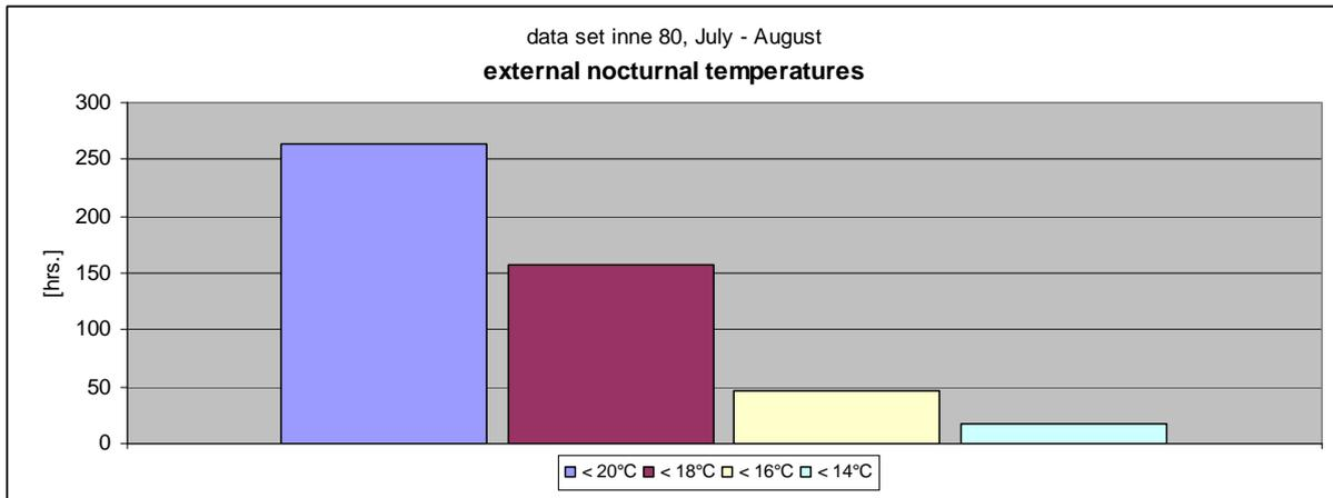
**Graph 45: Amount of hours with external nocturnal temperatures under-running various limits, data set "inne 80"**
