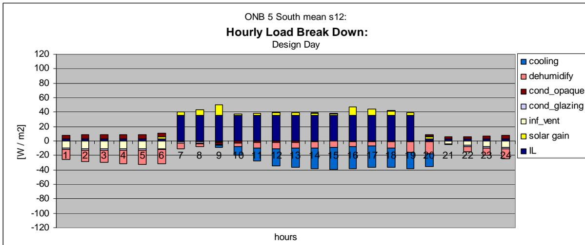
Graph 60: hourly gains and losses for ONB s12 (nocturnal ventilation)
