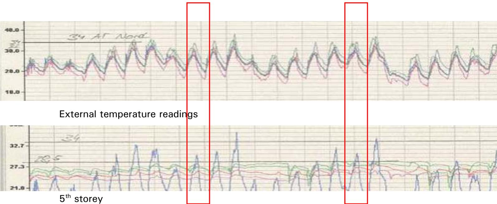
**Graph 52: Indoor air temperature observations (including outdoor air temperature: blue line; the red rectangles enframe the measurements of August 18 and August 27,2009, which are scrutinised against simulation results hereafter)**
