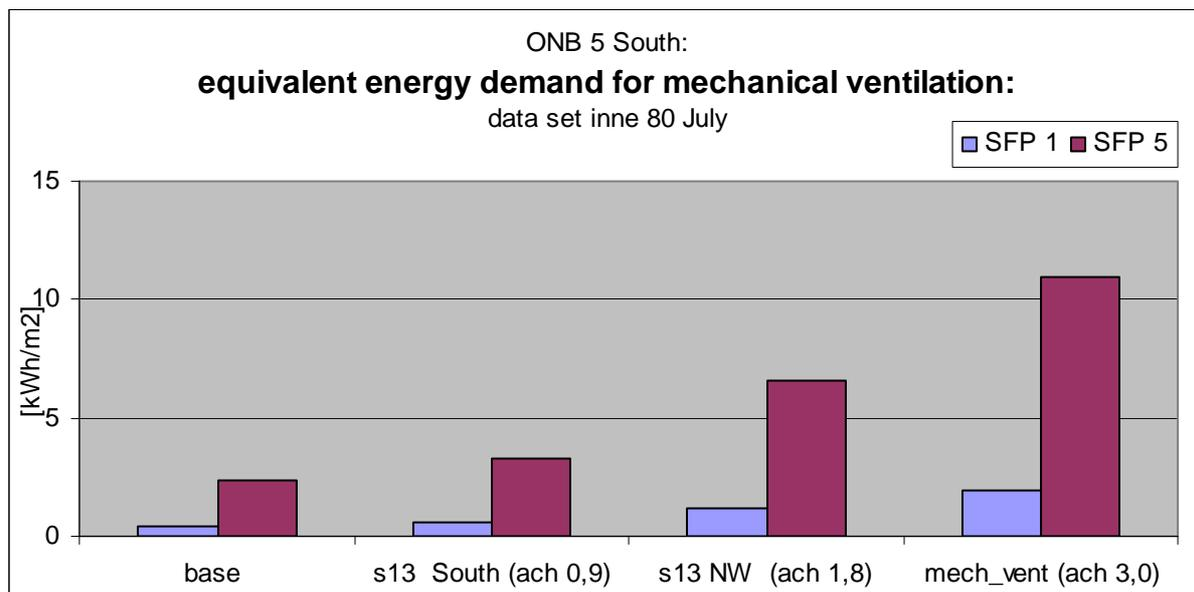
**Graph 71: Energy demand which would arise would natural ventilation be replaced by mechanical ventilation**
