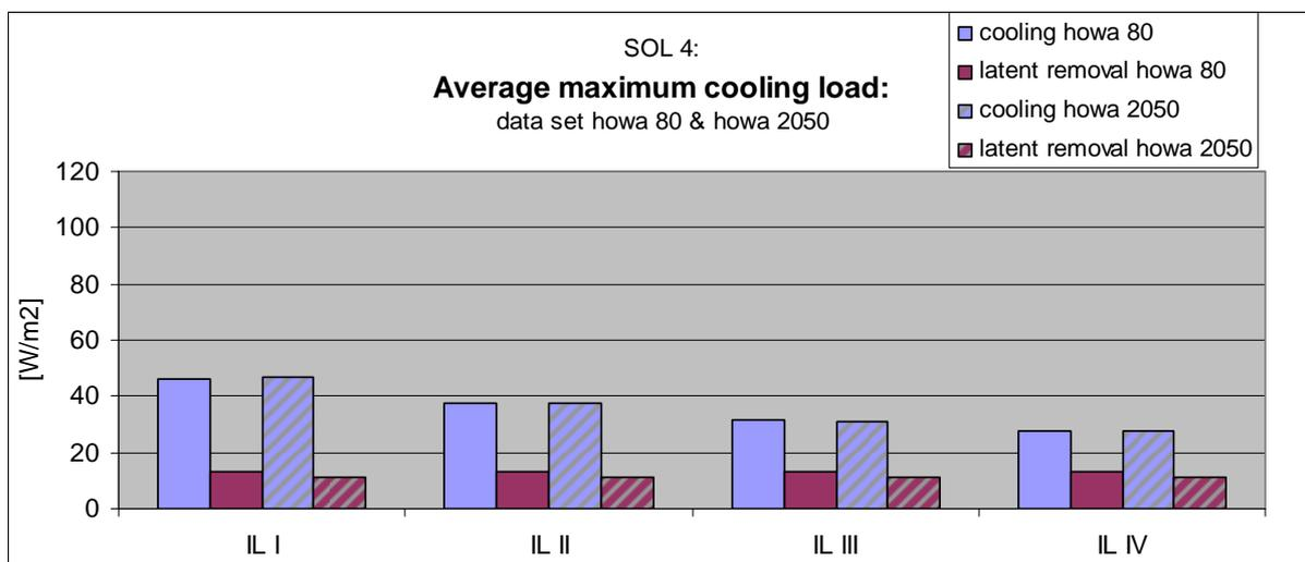
**Graph 29: SOL 4: maximum cooling loads for “howa 80” and “howa 2050” under different levels of internal load**
