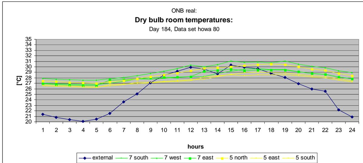
**Graph 54: Simulation results for a day comparable to August 27, 2009 (in terms of external temperature reached)**
