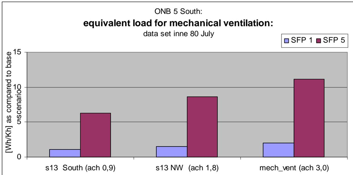
**Graph 72: Energy demand which would arise would natural ventilation be replaced by mechanical ventilation**
