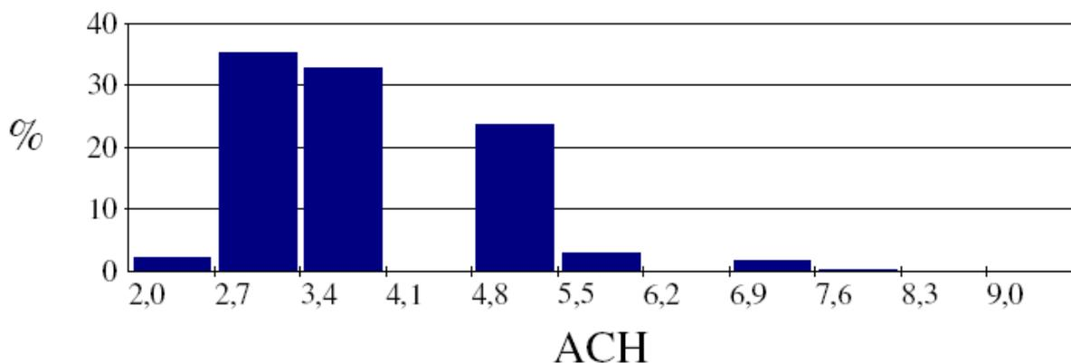
**Graph 59: Frequency Distribution of achievable air change rates due to natural ventilation for ONB s12 (nocturnal ventilation), wind direction South**
