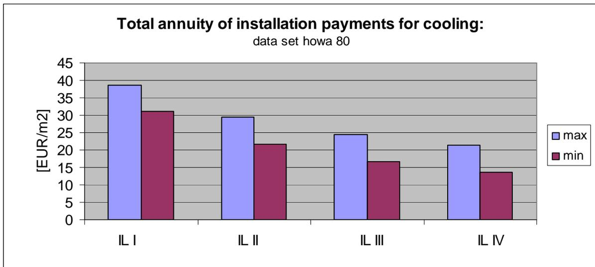
**Graph 82: Ranges of total annuity of installation payments under different levels of internal load for data set "howa 80":** values include annuities for investment, consumption and operation
