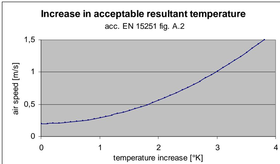
**Graph 77: increase in acceptable resultant temperature in dependence of air speed**
