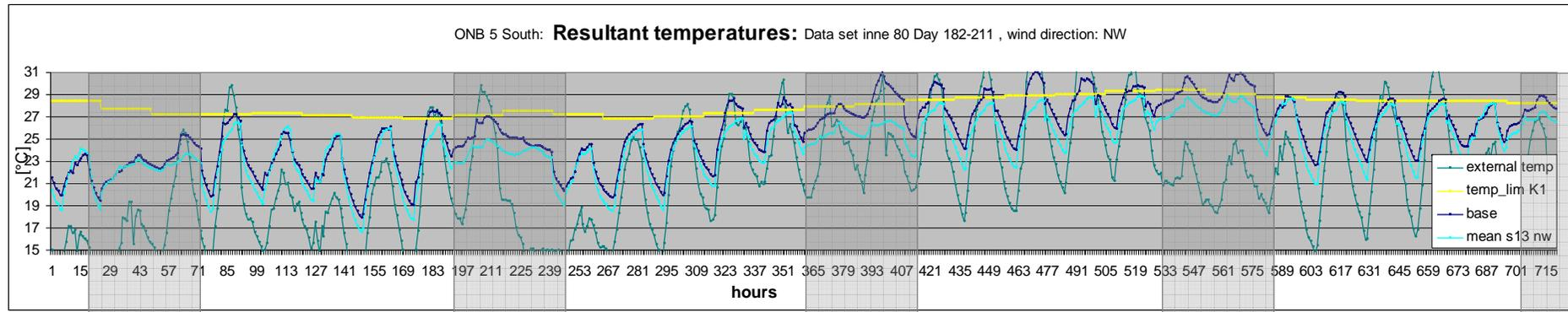
**Graph 68: Resultant temperature courses in ONB under base and s13 (extended nocturnal ventilation), wind direction NW; weekends are faded in grey;**
