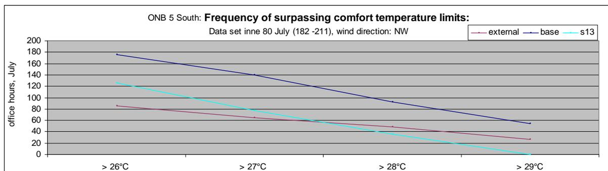
**Graph 70: Amount of hours during which temperature limits are surpassed in ONB under base and mechanical ventilation respective**
