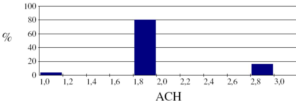
**Graph 63: Frequency Distribution of achievable air change rates due to natural ventilation for ONB s13 ( extended nocturnal ventilation), wind direction West**
