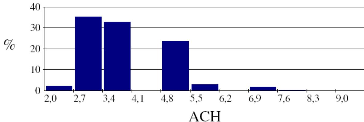
**Graph 58: Frequency Distribution of achievable air change rates due to natural ventilation for ONB s12 (nocturnal ventilation), wind direction West**
