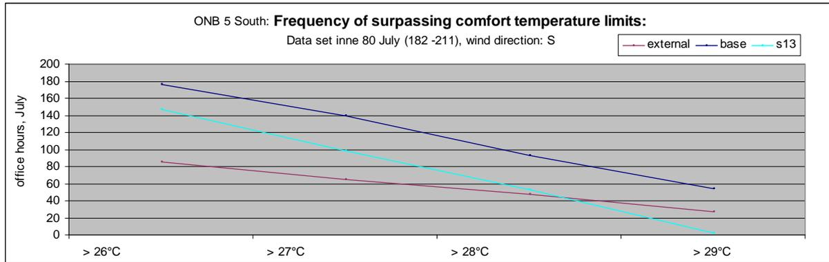
**Graph 67: Amount of hours during which temperature limits are surpassed in ONB under base and s13 (extended nocturnal ventilation) respective**
