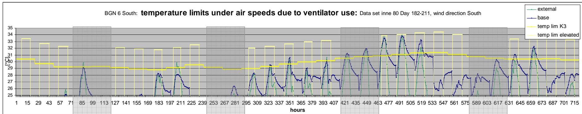
Graph 80: temperature limits due to fan induced air speed (acc. EN 15251) and outside temperature course
