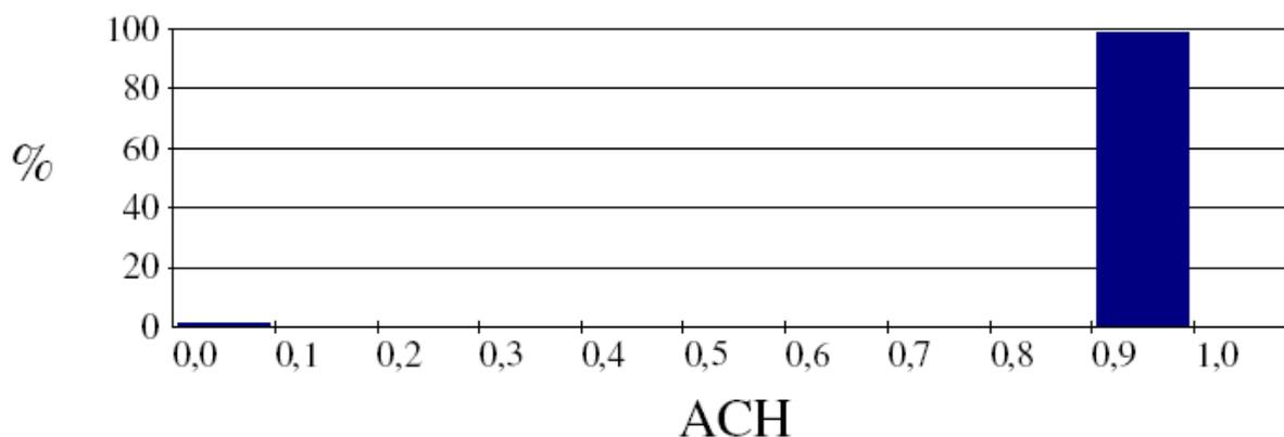
**Graph 64: Frequency Distribution of achievable air change rates due to natural ventilation for ONB s13 ( extended nocturnal ventilation), wind direction South**
