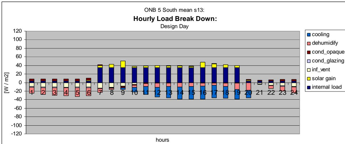
**Graph 65: hourly gains and losses for ONB s13 (extended nocturnal ventilation)**
