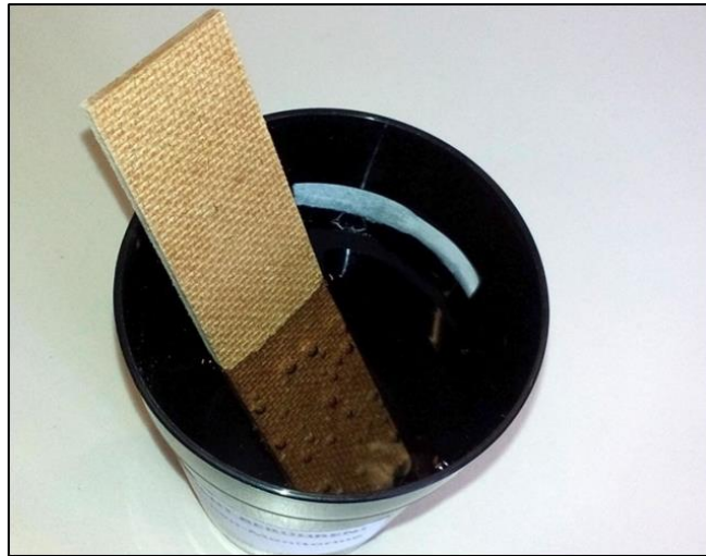
Fig. 5: The ovitrap is filled to about three-quarters (white line) with fresh tap water, and the wooden paddle is inserted with the rough side facing upward.
